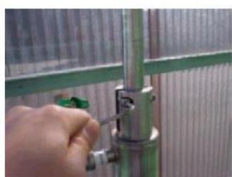
⑤Loosen the screw flow meter
